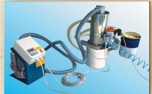
Caricamento automatico granuli Automatic granulates loading system
